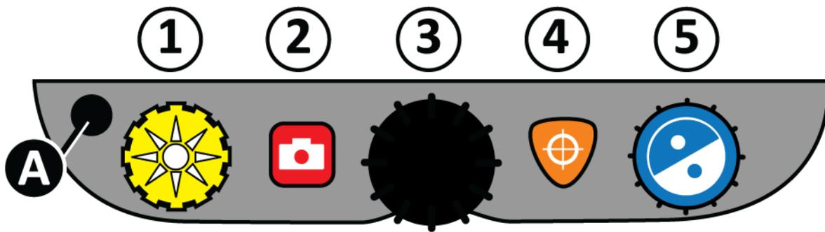
The black **ADVANCED** button (**A**) is used with other control panel buttons and dials to access and perform more features and operations.
