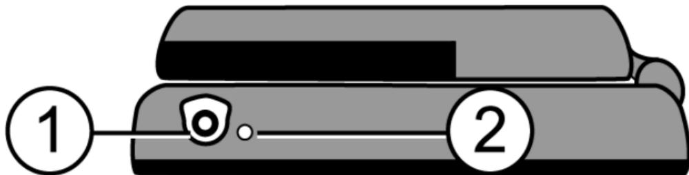
3. The LED stops blinking and glows a steady green once the batteries are charged. Unplug the power adapter from RUBY+. The battery LED turns off.
