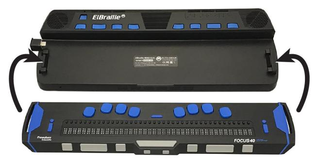
3. Push the locking lever to lock the display in place and establish the USB connection.
