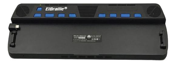
On the left side, going from the left front corner to the left back corner, you will find a lever for locking and unlocking the Focus Blue braille display. When you place a Focus Blue braille display into ElBraille, pushing the lever in locks the braille display in place. Pulling the lever out unlocks the braille display so it can be removed from ElBraille.
