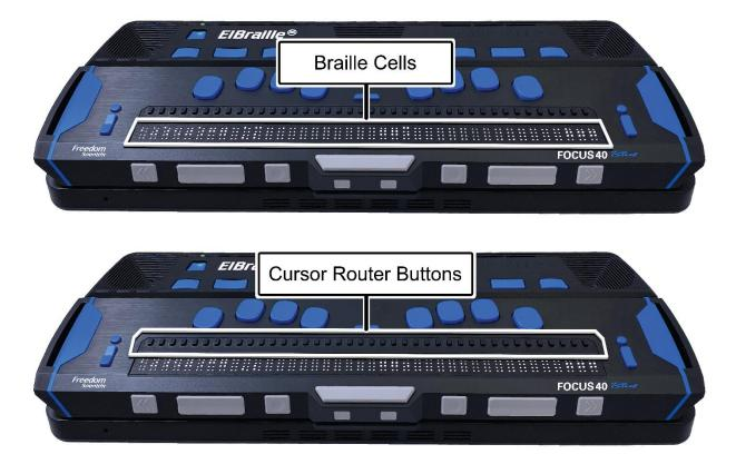
At each end of the display's surface are NAV Rockers used for easy navigation. Positioned above each NAV Rocker is a NAV mode button which cycles through different navigation modes.
