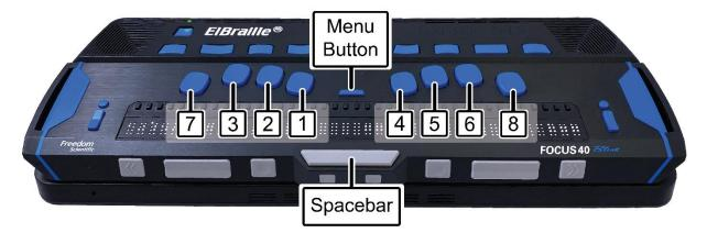
Between dots 1 and 4 is a Menu button which is used to access the Focus configuration menu as well as display Focus status information during an active connection.
