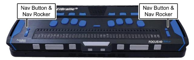
Positioned directly above the Cursor Router buttons is an 8-dot Perkinsstyle braille keyboard. Going from the center, the left-hand keys contain the following: Dot 1 under the index finger, Dot 2 under the middle finger, dot 3 under the ring finger, and dot 7 under the little finger, while the right-hand contains: Dot 4 under the index finger, Dot 5 under the middle finger, Dot 6 under the ring finger, and Dot 8 under the little finger. These keys are used to enter text or perform commands.
