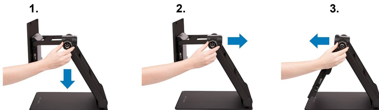
You can switch between modes by rotating/adjusting the camera using the Camera Positioning wheel (refer to ⑬ on pages 2 and 3).
